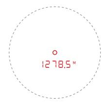
b. Golf Mode: In a group of targets, hold the button while aiming at the target for scanning. The nearest target is locked first. The values displayed on the screen do not change (nearest distance).
