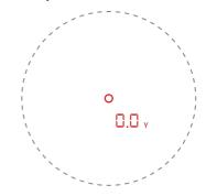
2. Menu select: Long press M button for 2 seconds to enter the mode setting menu. Using the D button you can scroll through the icons. Short press button to advance to the next screen. In mode setting menu long press M button for 2 seconds to return to ranging display.
