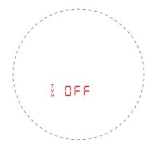
a. LOS mode (OFF): Aim the reticle at the target. Short press button once to measure the distance. Only the linear distance of the ranging is displayed.
